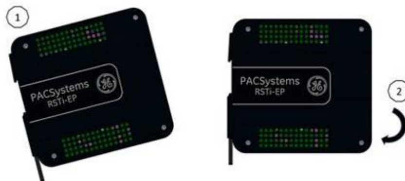
Figure 237: Mounting positions of the EPSCPE100/CPE115 on DIN rail
